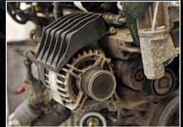
*Alternators can suffer from water ingress, resulting in seizure or even the casings splitting in two*
