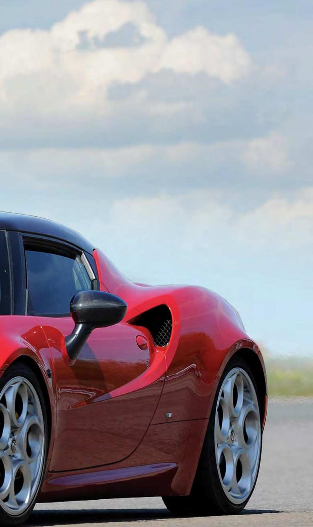
machines, but the 4C was the real deal. There was nothing second-rate about its specification. The carbon central tub weighed just 107kg, and while Alfa Romeo quoted an overall dry weight of just 895kg for the car, a more realistic kerb weight figure was around 1100kg. Not everything was carbon: aluminium was used for the subframes front and rear, while the outer body was in composite (claimed to be 20 per cent lighter than steel).
