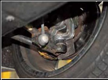
*If front ball joints are creaking, investigate immediately. If they fail, you can lose a wheel*
