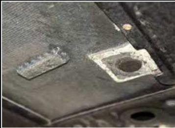
*Carbon tub does have some metal elements in it. Check very carefully for any signs of accident damage*
